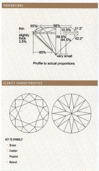
\* Red symbols denote internal characteristics (inclusions). Green or black symbols denote external characteristics (blemishes). Diagram is an approximate representation of the diamond, and symbols shown indicate type, position, and approximate size of clarity characteristics. All clarity characteristics may not be shown. Details of finish are not shown.
